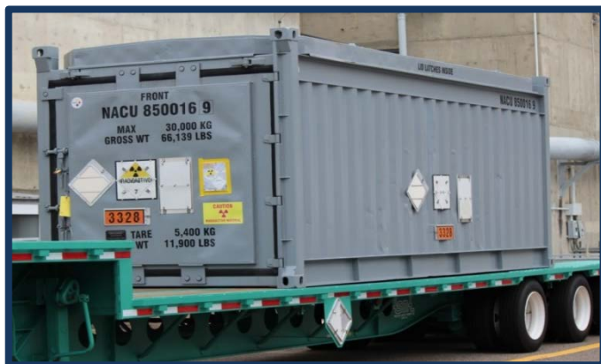
International Standards Organization (ISO) Container containing a Legal Weight Truck (LWT) Cask
