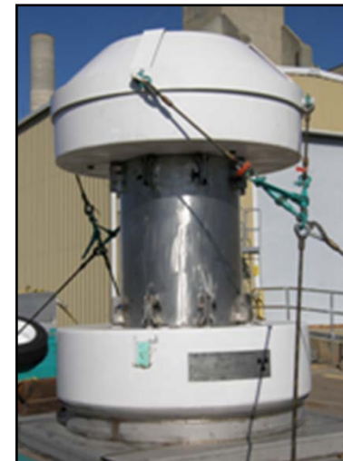
Decon, Reassembly & Ship Empty Cask
