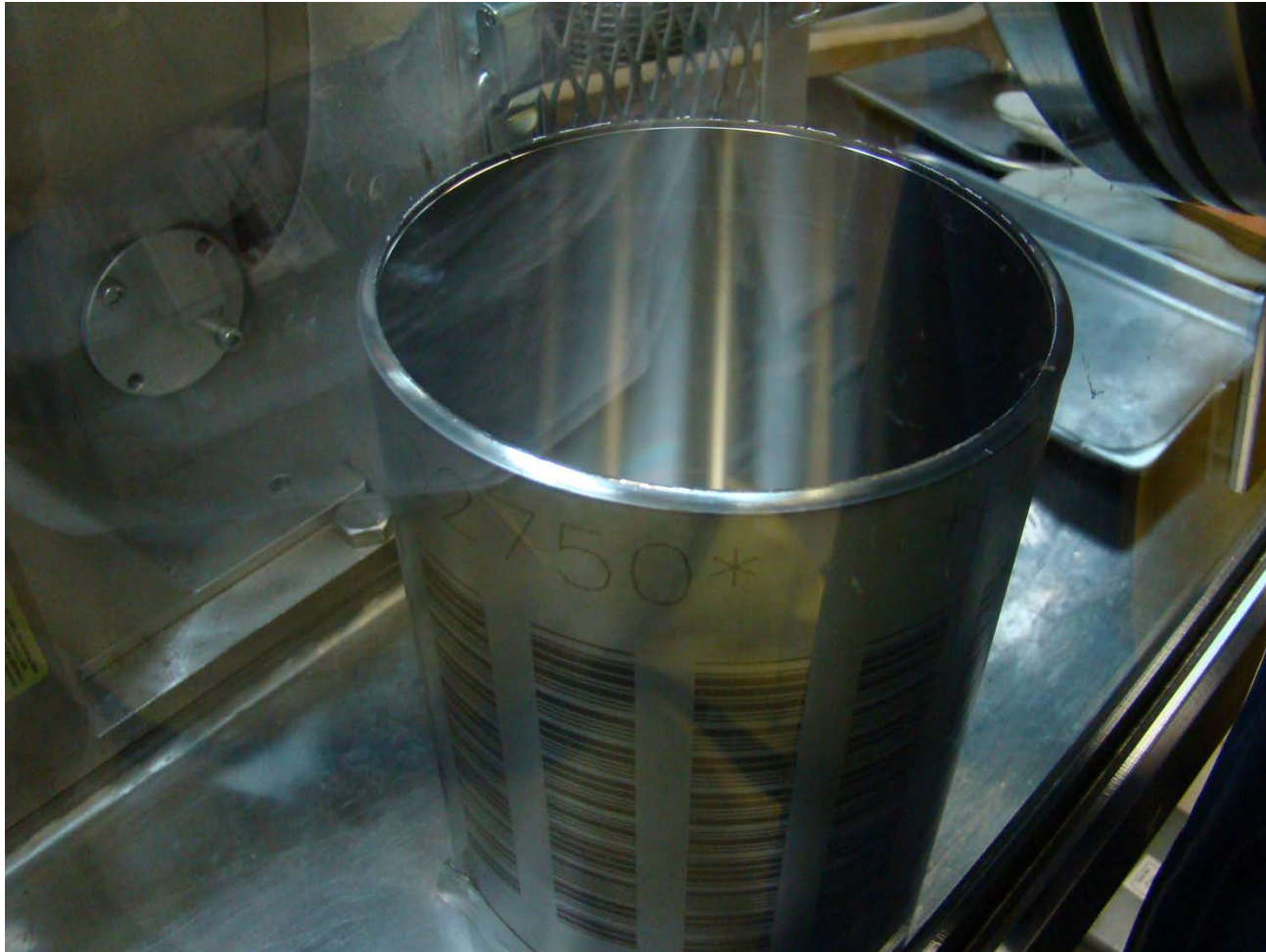
3013 Container Cut for Oxide Removal and Metallurgical Examination
