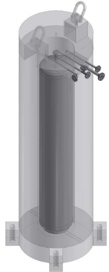
Shielded Ion Exchange Column (Dimensions 12'x5.5' Shielded)
